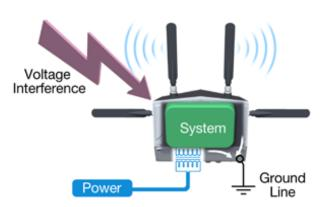
wireless devices can also be galvanically isolated to provide total isolation of internal device circuitry and further protection from electromagnetic disturbances.
