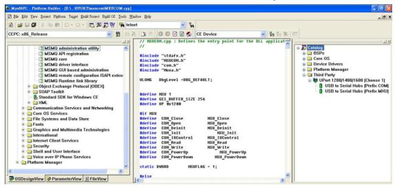
3. Right-click on the driver "USB to Serial Adaptors (Prefix COM)" or "USB to Serial Adaptors (Prefix MXU)" and then choose "Add to OS Design." After adding the driver, you should be able to find it in your workspace. At this point, you can start building your operating system and download it to a target.
