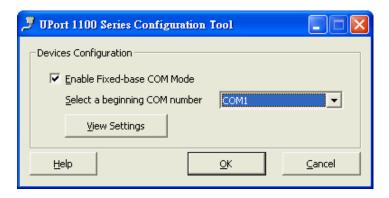
The COM numbers are assigned sequentially, and are not tied to a specific UPort device or USB port number. For example, let's assume that you've set COM1 as the first COM number that will be assigned. If a UPort 1150 is plugged into your computer's USB port 1, your computer assigns COM1 to the UPort's serial port. When the UPort 1150 is plugged into USB port 2, the computer still assigns COM1 to the UPort's serial port.
