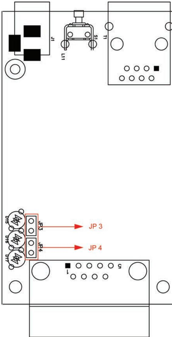
To set the pull high/low resistors to 150 K $\Omega$ , leave jumpers JP3 and JP4 open (not shorted). This is the default setting.
