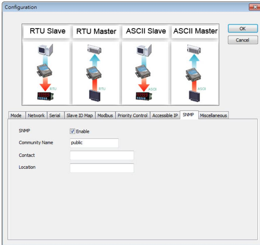
To enable the **SNMP** function, select the **Enable** checkbox.
