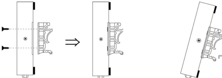
**Mounting on the wall:** Place two screws in the wall and slide the unit onto the screws as shown. The head of each screw 6.5 mm or less in diameter, and the shaft should be 3 mm or less in diameter. Make sure to leave about 2 mm of space between the head and the wall.
