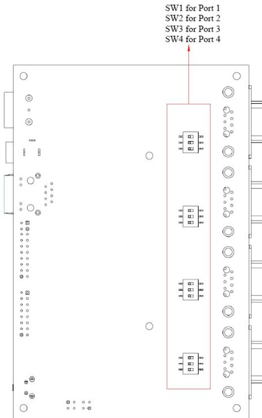
**To add a 120 Ω termination resistor**, set switch 3 on the port’s assigned DIP switch to ON; set switch 3 to OFF (the default setting) to disable the termination resistor.
