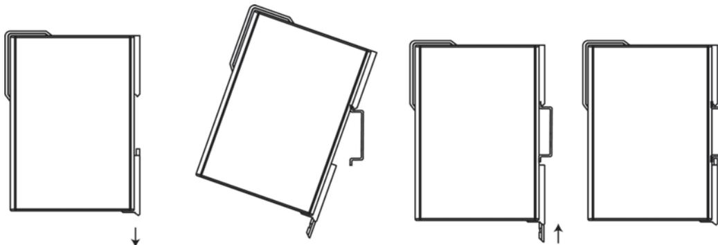
**Mounting on the wall:** Pull out both the top and bottom sliders and align the screws accordingly.
