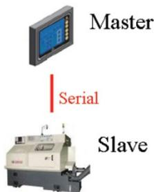
An advanced multiport MGate model (MB3270) can be inserted into the serial system, with the slaves connected to one serial port and the master to another serial port. The advanced gateway allows Ethernet masters to communicate with the serial slaves, and it also provides a serial redirector function that simultaneously allows the serial master to continue controlling the slaves.
