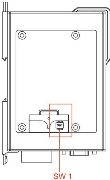
The DIP switches are located beneath the DIP switch panel on the side of the unit.
