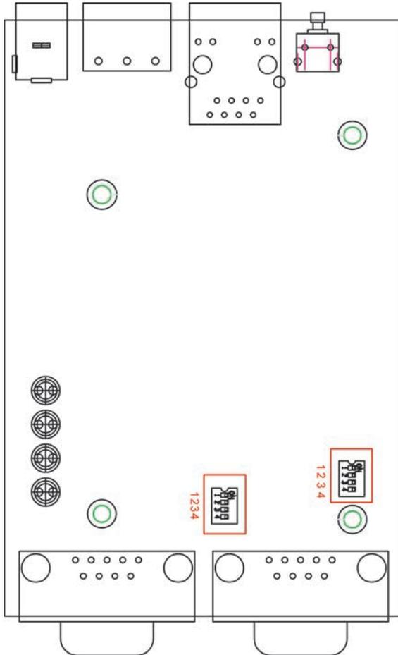
**To add a 120 Ω termination resistor**, set switch 3 on the port's assigned DIP switch to ON; set switch 3 to OFF (the default setting) to disable the termination resistor.
