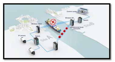
2. Frequency-Interference Failover: This concept is similar to the previous model. If the communication frequency experiences interference and data can no longer be transmitted over the Active frequency, it will resume the connection via another Backup frequency.
